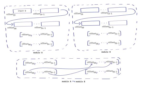
Figure 11: Composing AA modules A and B into an audio graph
