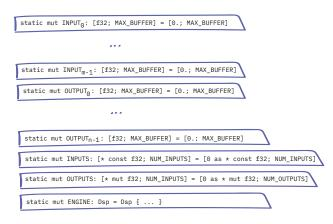
Figure 9: AA module static memory layout.
